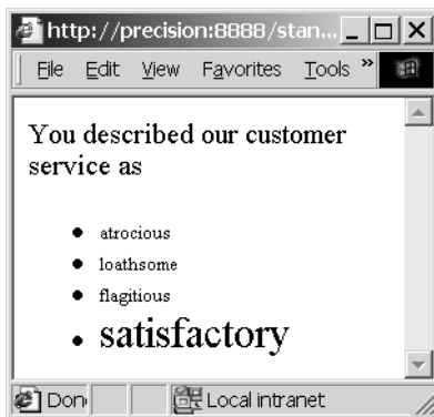
Figure 11.3 The checkbox2.jsp page from listing 11.3 looks at individual parameters' values before printing them out. In this case, the page glorifies positive remarks by printing them in large letters; it similarly diminishes negative feedback by making it smaller.
