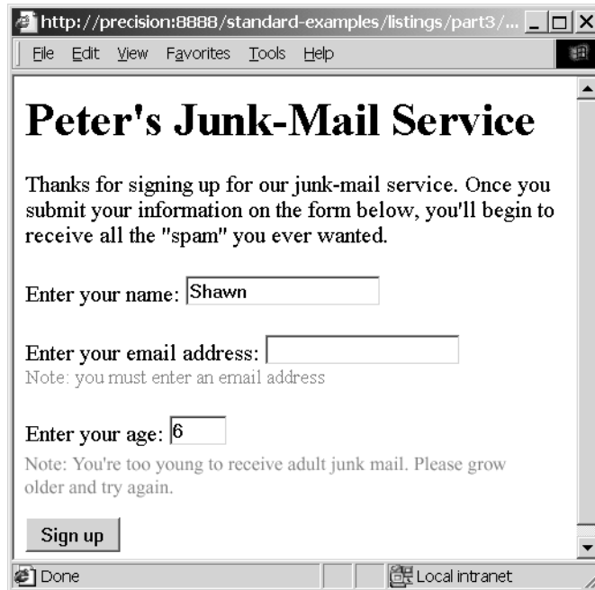
Figure 11.12 When the page from listing 11.9 is fed invalid input, it reprints its form with appropriate error messages interspersed. It also explicitly fills in the form with the values the user entered, making it easier for the user to correct them.
