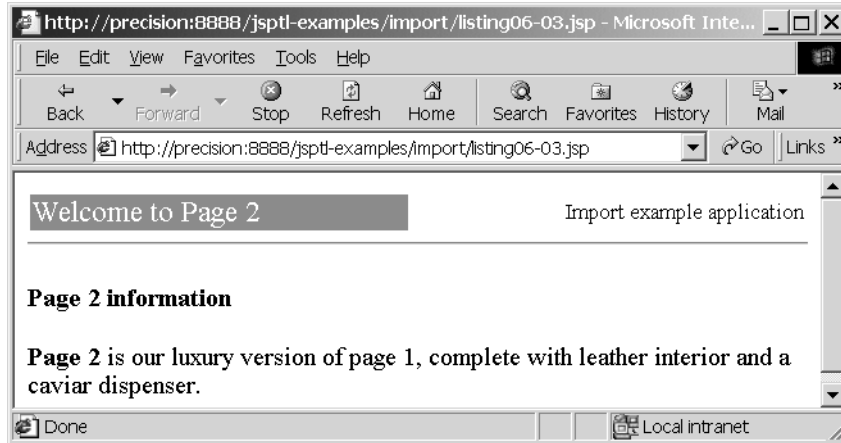
Figure 6.7 A web browser's display of page2.jsp , which supplies the text "Welcome to Page 2" to the header page. Note how the static text and form of the header are unchanged from page1.jsp ; only the parameterized text differs.
